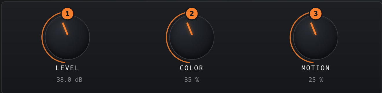
FIG. 3 - LANE MACRO ROW. IN LINKED STEREO THERE IS ONE SET; IN L/R OR M/S THERE ARE TWO STACKED LANES.
