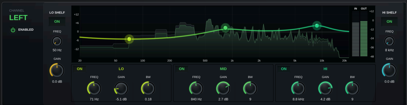
FIG. 3 — CHANNEL STRIP, LEFT. SAME LAYOUT FOR RIGHT (DIFFERENT COLOURS) AND FOR MID/SIDE IN M/S MODE.
