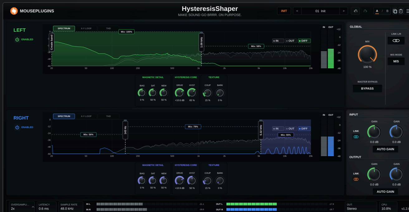
FIG. 4 - MULTIBAND WINDOW IN INDEPENDENT L/R MODE. EACH LANE SHOWS THREE BANDS SEPARATED BY TWO CROSSOVER HANDLES, A MIX MARKER PER BAND, AND A BAND-TINT BEHIND THE ACTIVE BAND.
