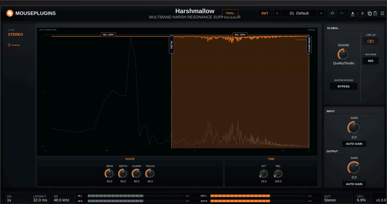
FIG. 1 - HARSHMALLOW IN LINKED STEREO (LINK L/R ON), SHOWN WITH THE LOW/MID CROSSOVER DRAGGED IN TO 543 HZ (LO + MID BANDS). ON FIRST LOAD BOTH CROSSOVERS SIT AT THE CHART EDGES FOR A SINGLE FULL-RANGE BAND.
