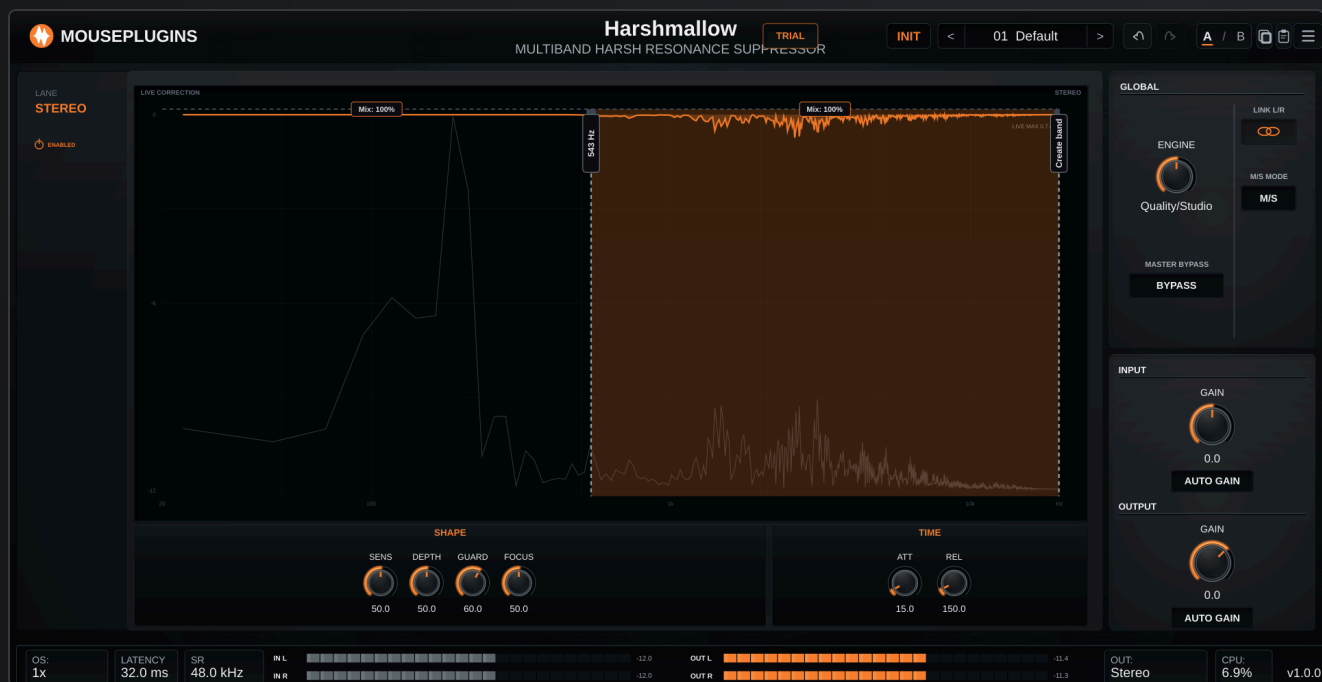
FIG. 3 - THE LANE CHART. FREQUENCY RUNS LEFT TO RIGHT (20 HZ TO 20 KHZ); THE VERTICAL AXIS SHOWS REDUCTION IN DB (0 AT THE TOP, DOWN TO -12).
