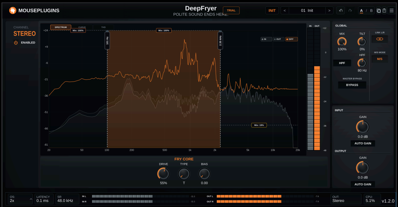
FIG. 2 — THREE BANDS SPLIT: TWO CROSSOVER HANDLES DRAGGED INWARD, THE MID BAND TINTED, FREQUENCY PILLS AND PER-BAND MIX MARKERS VISIBLE
