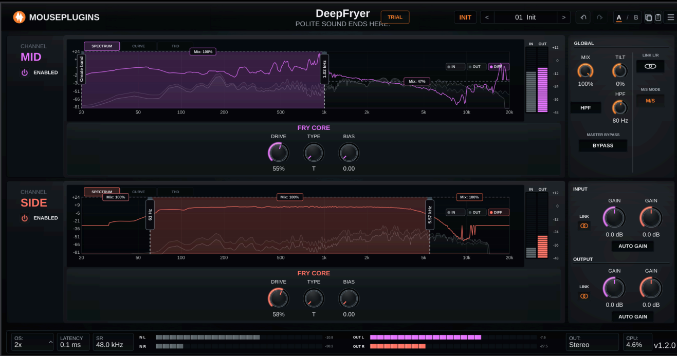
FIG. 3 – MID/SIDE ROUTING: TWO STACKED LANES, MID IN PURPLE AND SIDE IN RED, EACH WITH ITS OWN CHART AND FRY CORE
